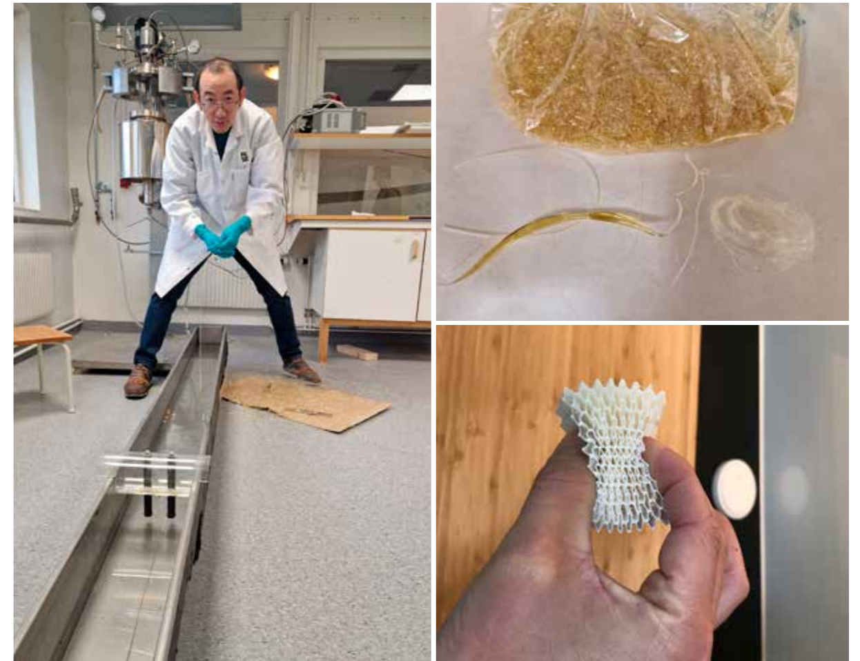
Left image: Zengwei Guo (RISE) is collecting PBF fibers during a large scale experiment in Mission 2. Top right image: PBF filaments and pellets. Lower right image: Miniature model of 3D-printed foam produced in Mission 4.
