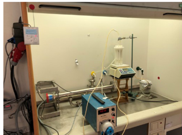
FIGURE 17. Setup of biofilm reactors to analyze parallel surfaces. The setup consists of three parallel reactors, where the rotor speed can be differentiated, and a unit for decontamination of water, if pathogens are present.
